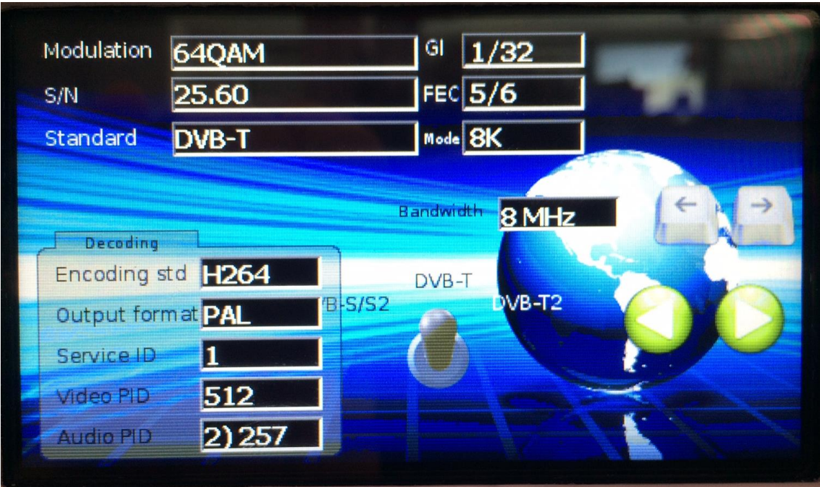
FIGURE 99: RECEIVING HEAD – DEMODULATION AND DECODING CONFIG.
