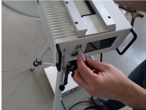
FIGURE 29: BOOSTER POWER SUPPLY CABLE CONNECTION A
